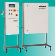
Intellimix 3: Electronically controlled two-component dosing system
