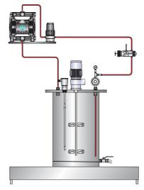
Connection diagram: low-pressure circulation system
