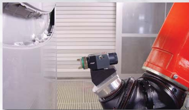
All variations in the SATA LP jet K3 line are available for robotic use.
