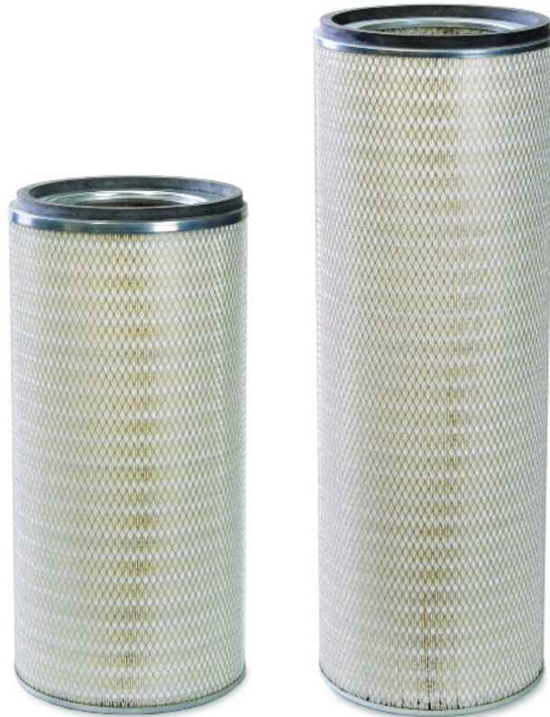
Electro-galvanized inner and outer screens of 26" and 36" filters have 75-percent open area for maximum air flow and powder release.
