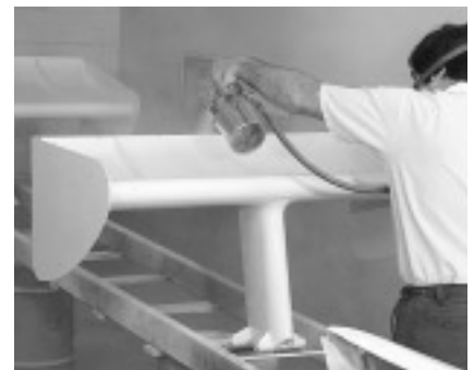
JGA-HVLP suction feed provides high quality atomization with the high transfer efficiency of HVLP.
